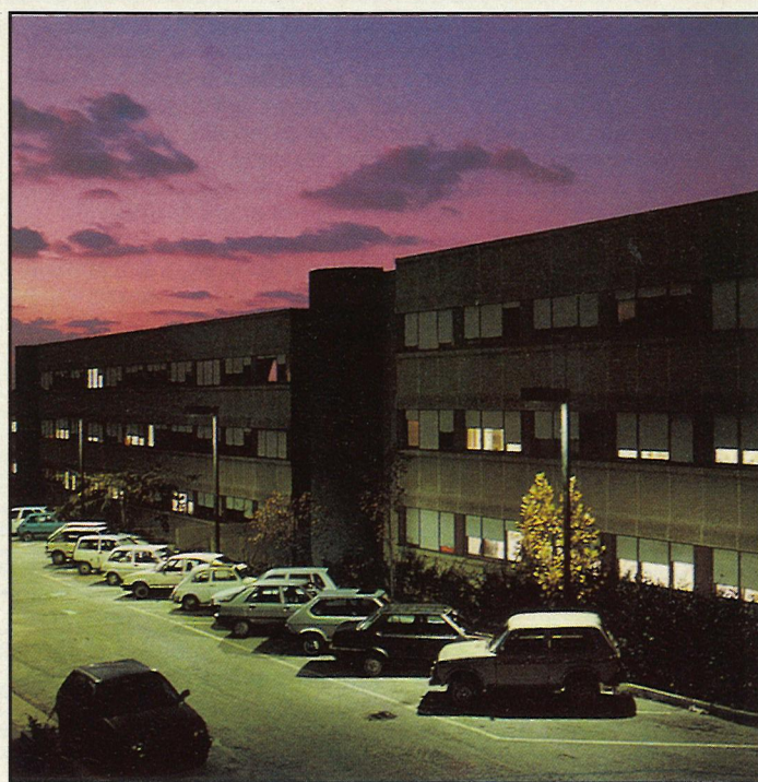
A typical Asymmetric Cut-Off Luminaire in use. Note that the light is being thrown on to the car park as required and not the building.
