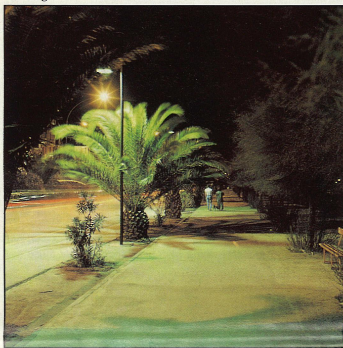
With the distribution of this reflector (fig 4) the light is directed more towards the pathway than the roadway.
